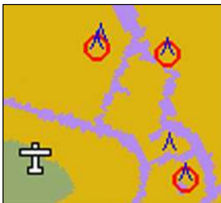
Figure 24: Blow-up of Map Display showing terrain and obstacle warnings. The Yellow terrain and the tips of the blue obstacles are within 2000 feet of the aircraft's altitude. The red-circled obstacles are at or above the aircraft's altitude.
