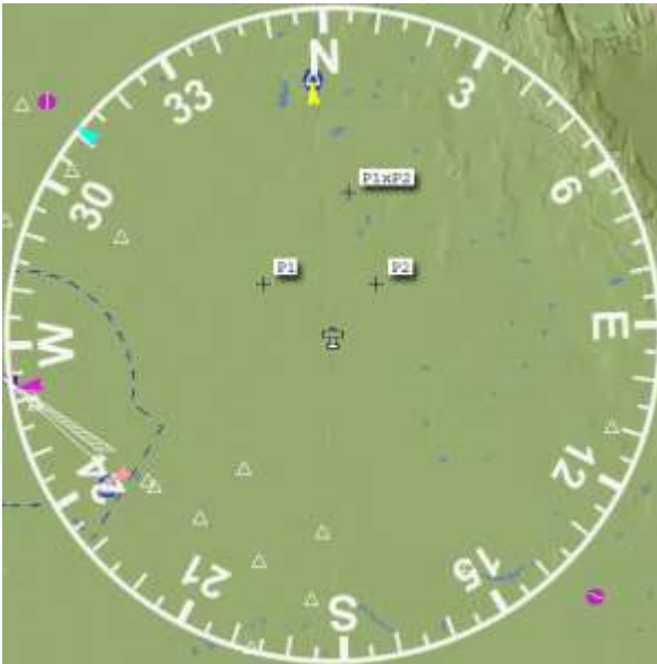
Figure 27: Triangulation example, showing triangulated waypoint P1xP2 triangulated from User Waypoints P1 and P2.
