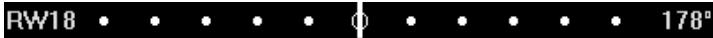
Figure 7: Using the Course Deviation Indicator (CDI) for the runway approach RW18. Note that the white needle is lined up with the center point of the indicator, and that the OBS is 178 degrees. If the needle is red on either side of the indicator, then that means that the airplane is more than 3° off the center of the course.
